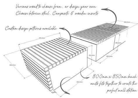
Manufactured from mild steel, e-coated and powder coated. Also available in a stainless steel finish
